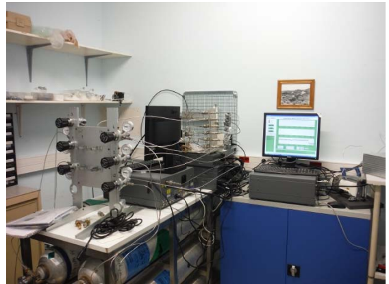
Experimental set-up for measuring greenhouse gas concentrations. © O. Llido
