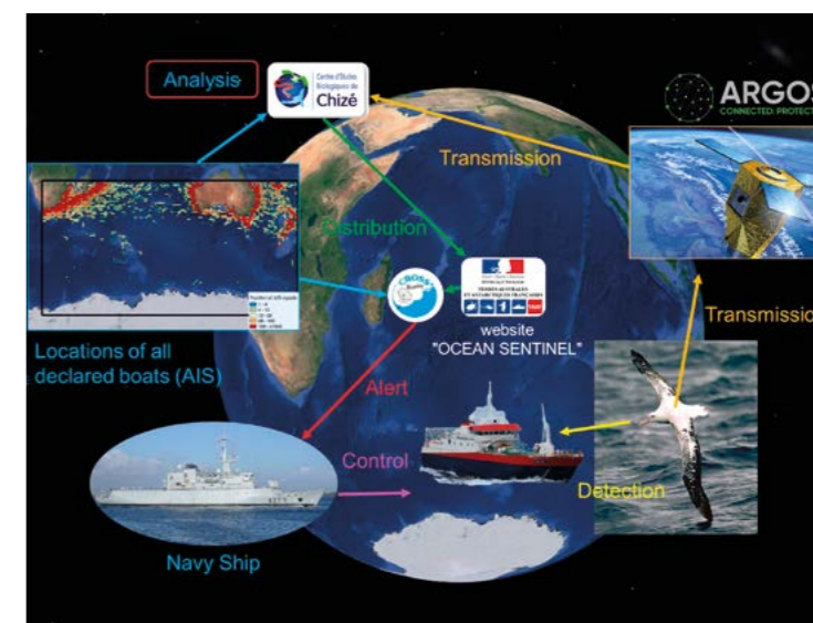
Figure 4 - Diagram of the Ocean Sentinel concept, detection by Centurion, transmission by Argos system, Data analysis and integration of AIS data, provision of data on the TAAF website and alert in case of detection of undeclared activity, with potential intervention if a French Navy vessel is in the area.
