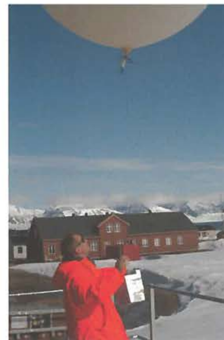
▲ Start of a balloon with an ozone radio sonde (photo: M. Herrmann)
