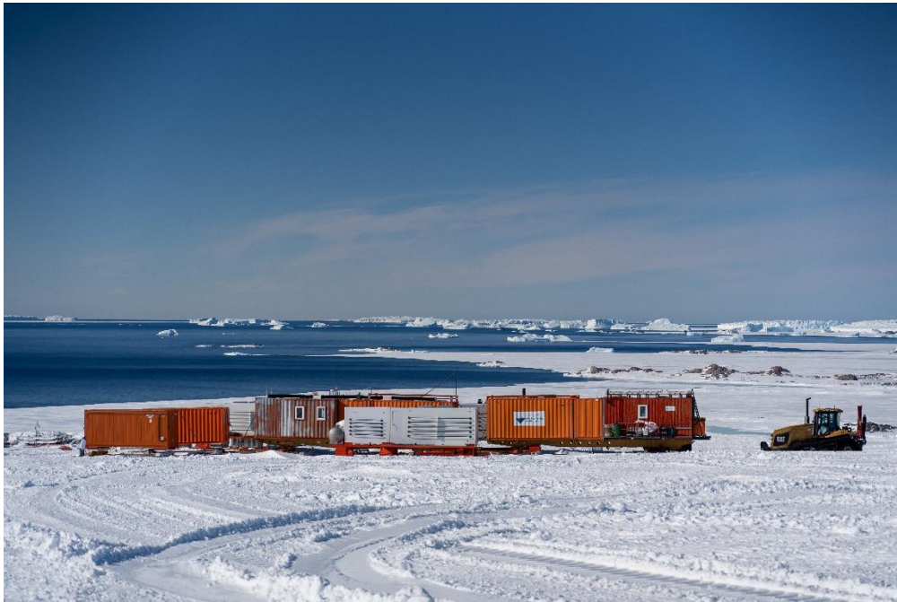
Departure of the AWACA convoy from the Adélie Coast. The sledges which carry the observation units, the living unit for the personnel and the fuel reserves are hitched to the tractors that will take them to the project's various observation sites. © Nicolas Pernin / French Polar Institute
